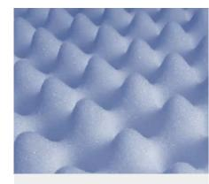
Polymers and foams Gas pycnometry is widely used to characterize the relative amounts of crystalline and amorphous phases within polymer materials. This technique is also used to assess the open cell content of foam materials to predict their performance as insulators or as sound- or collision dampening materials.
