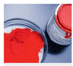
Powder coatings and dried film coatings The crystallinity of plastics and the true density of dry pigments are monitored by gas pycnometry to better understand the mechanical behavior of these materials. In addition, gas pycnometry can help determine the volatile organic content within dried films in order to assess the level of curing.
