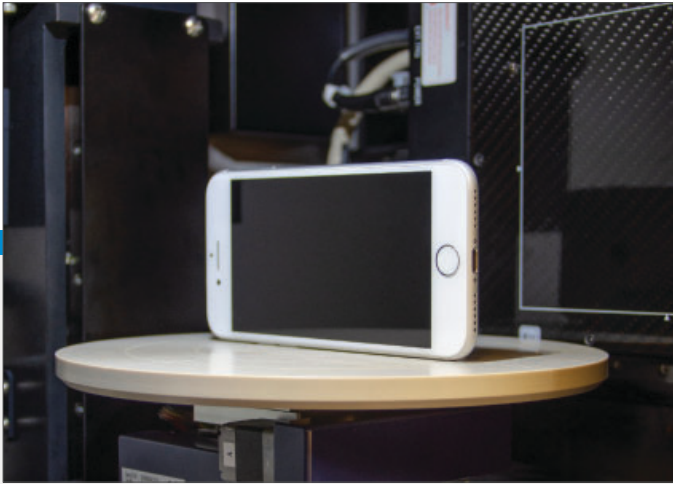
Large sample stage with smartphone and view of flat panel detector
