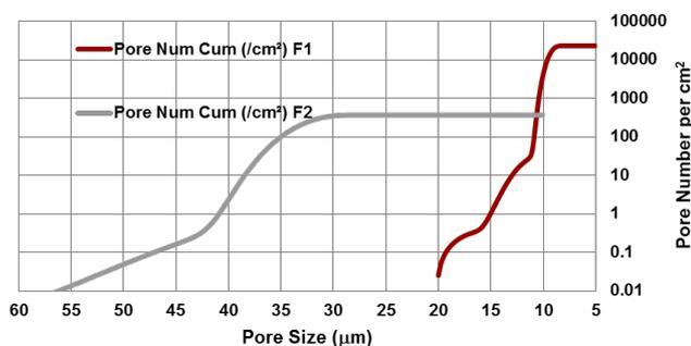
Figure 5: Cumulative pore number per unit area versus pore size.
