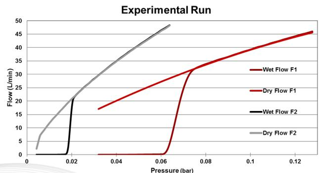
Figure 3: Measured flow rate versus pressure for the two filters F1 and F2.
