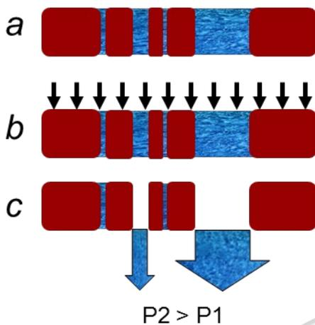
Figure 1: (a) A completely wetted sample (b) experiences a gas pressure from the upstream to the downstream which (c) forces the wetting fluid from the larger pores (P1) then to the smaller pores (P2) as the pressure increases.
