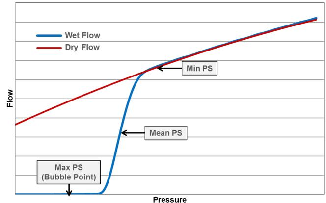
Figure 2: Characteristic wet and dry curves showing the locations of the maximum, mean, and minimum pore size.
