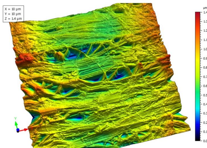
Figure 4:  $10 \times 10 \mu\text{m}$  3-D topography (forward trace) AFM image of the PTFE tape surface showing fibrous composition of the tape.
