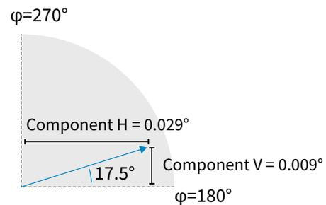
Figure 3. Measured offcut orientation and components of NIST SRM 1995 Al<sub>2</sub>O<sub>3</sub> wafer
