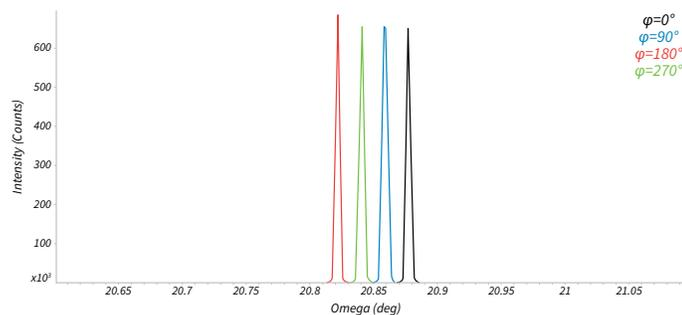
Figure 2. Overlay plot of the four Omega scans for the NIST SRM 1995 Al<sub>2</sub>O<sub>3</sub> wafer
